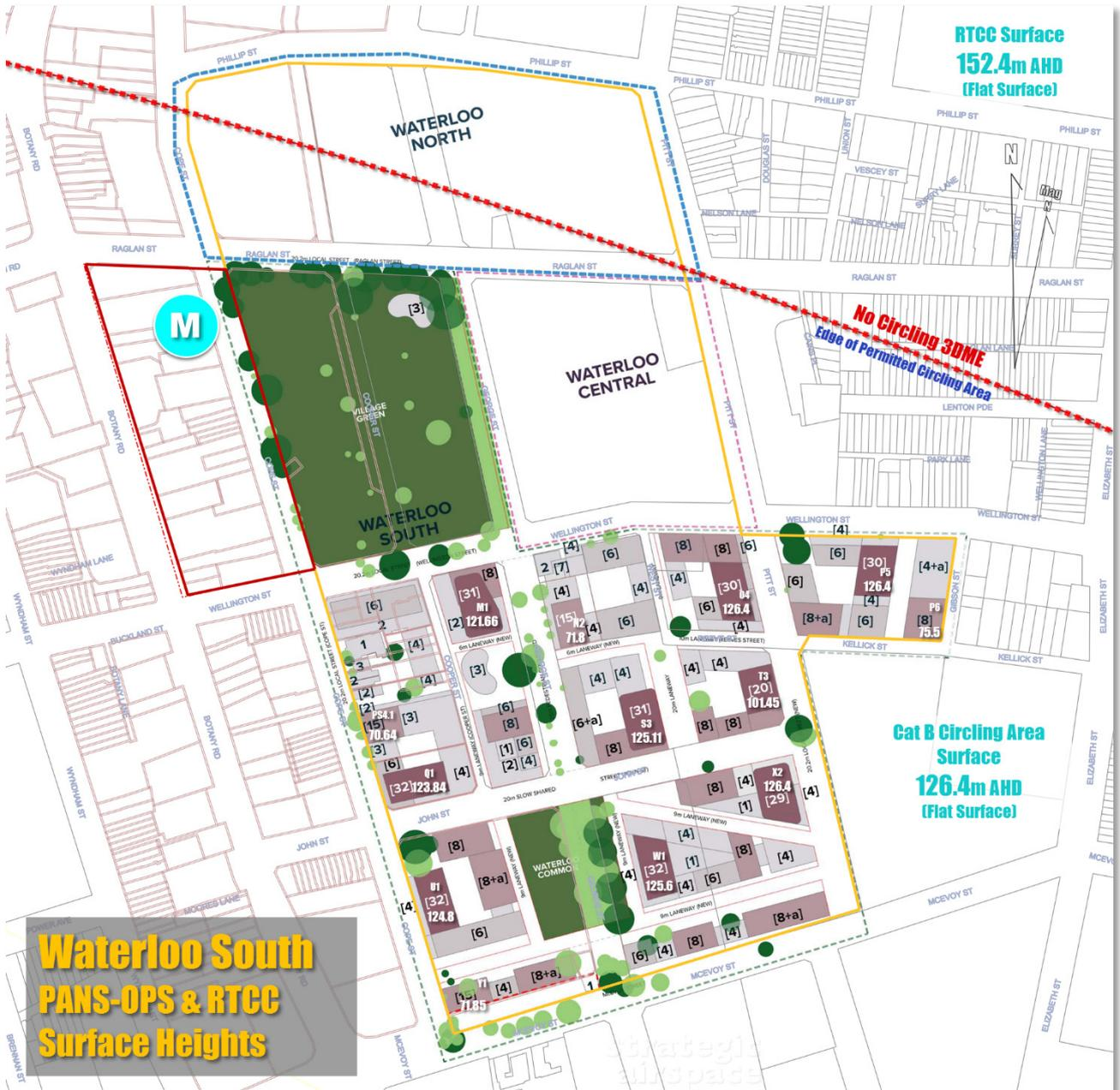
Figure 9 — PANS-OPS & RTCC/MVA Height Constraints across the Waterloo Precinct
